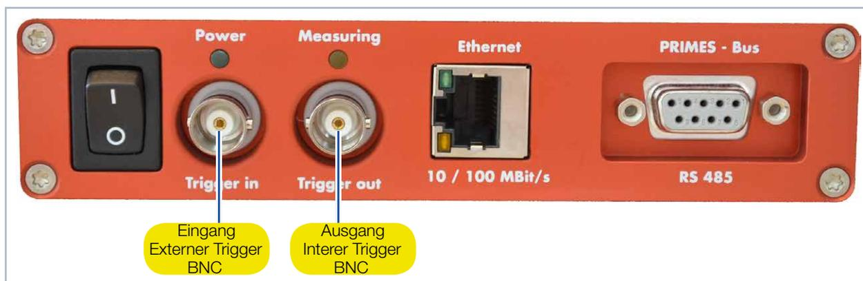
Abb. 12.14: Triggeranschlüsse
